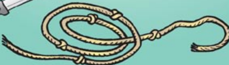
A 5 m length of measuring rope
