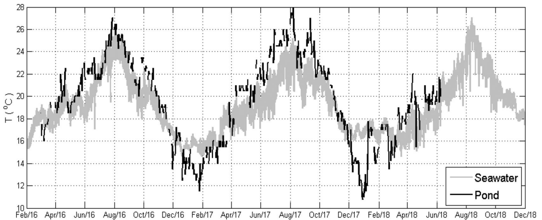
FIGURE 2 Sea water temperature in ponds and surface ocean temperature from February 2016 to December 2018 (data obtained from www.redmar.cicese.mx ). The temperature within the ponds is the daily average obtained from maximum/minimum thermometers
