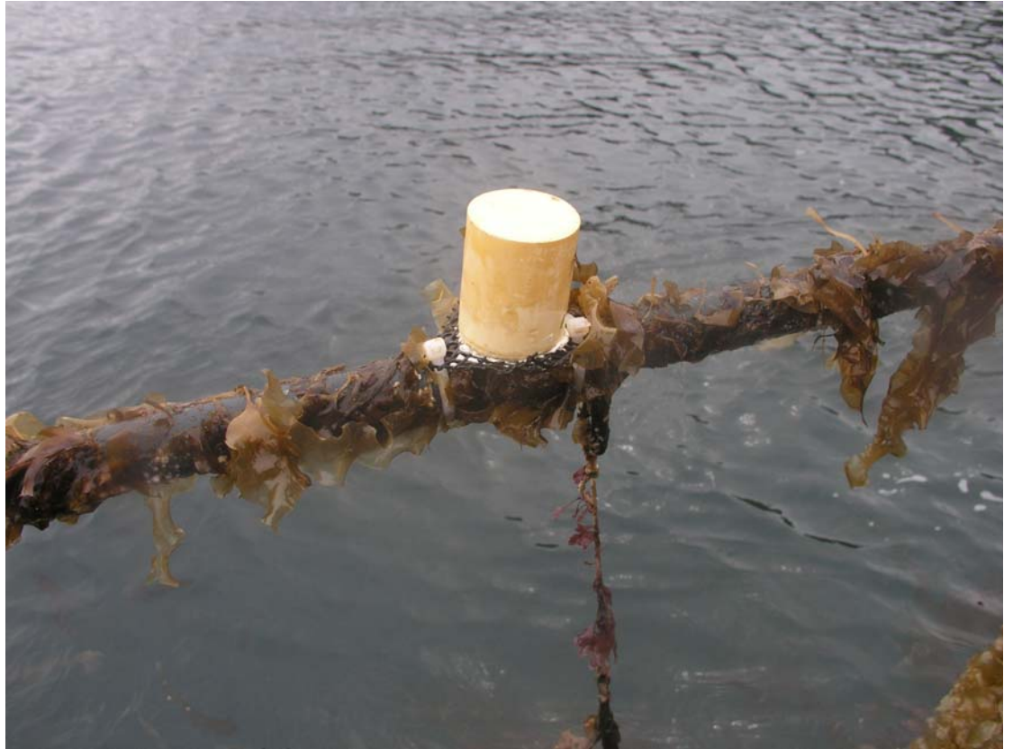
Figure 5.4 Plaster cylinder facing upwards on top of buoyed frame at deployment.
