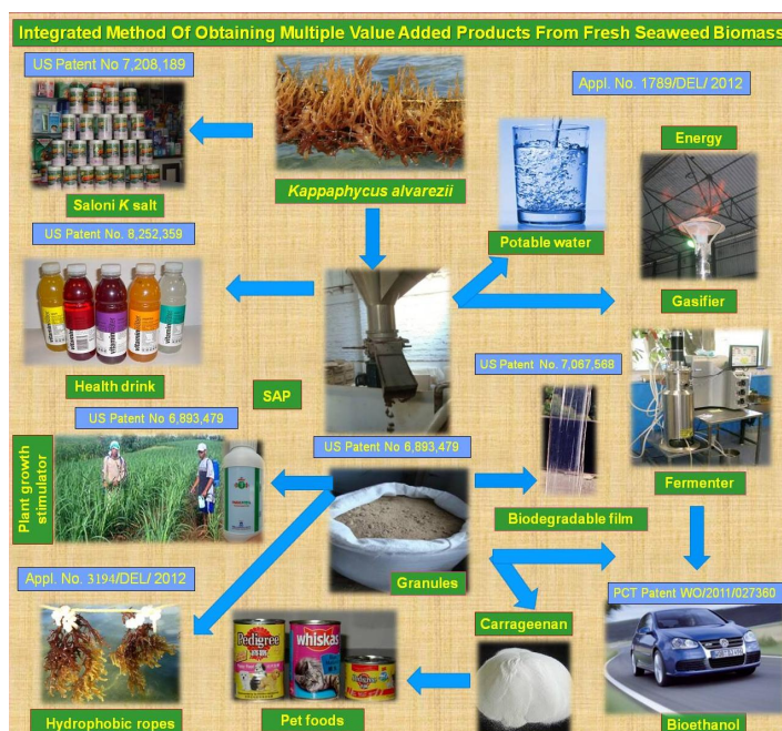
Fig : 4. Integrated process producing multiple products from Kappaphycus
