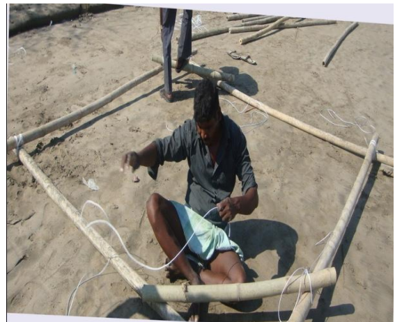
Fig : 7 Fabrication of bamboo raft
