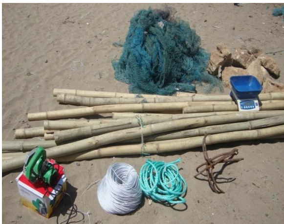
Fig : 6 Material required for fabrication and transplantation of the bamboo raft in the sea
