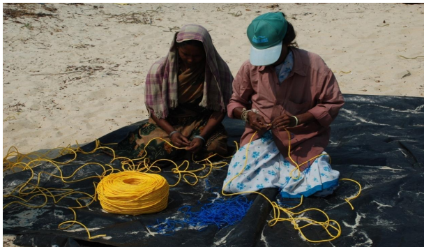
Fig : 9 Insertion of loops between braiders of seeding rope
