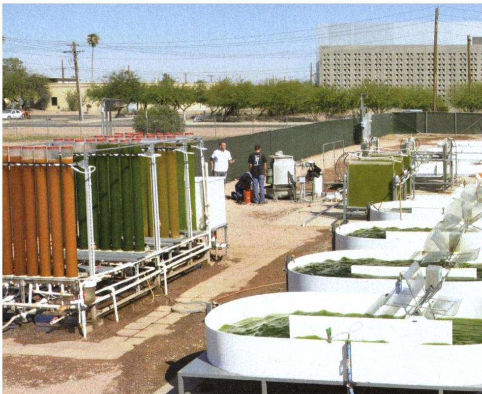
Figure 5. Arizona State University is evaluating multiple algae-cultivation systems, including the open ponds, tubular photobioreactors and flat-panel photobioreactors above. The differently colored cultures contain different algal strains or the same strain grown under different culture conditions. (Photograph courtesy of Qiang Hu of Arizona State University.)
