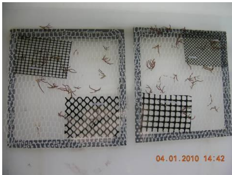
Figure 9. Test Panels of Polyester Netting and Plastic Aquaculture Mesh with Pieces of Gracilaria pacifica Entangled into Mesh
