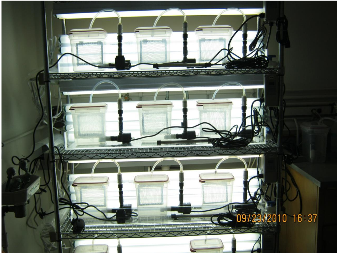
Figure 10. Twelve-Place, 4-Tier Mini-Spray Culture System (UCSD-SIO)
