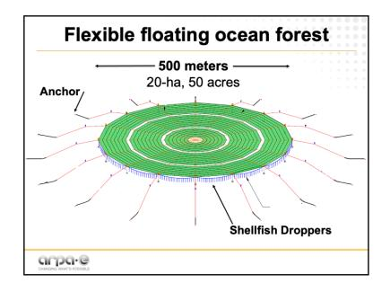
This is the Spiderweb, a depth adjusting reef we have developed for the Department of Energy. The green area provides a substrate for growing seaweed, finfish shelters, and hanging shellfish. The substrate is normally 2 to 6 meters deep when growing *Gracilaria Tikvahiae* in the Gulf of Mexico. If a storm approaches, the entire structure submerges to at least 40 meters deep. The system is designed for seafloor depths between 50 to 100 meters.
