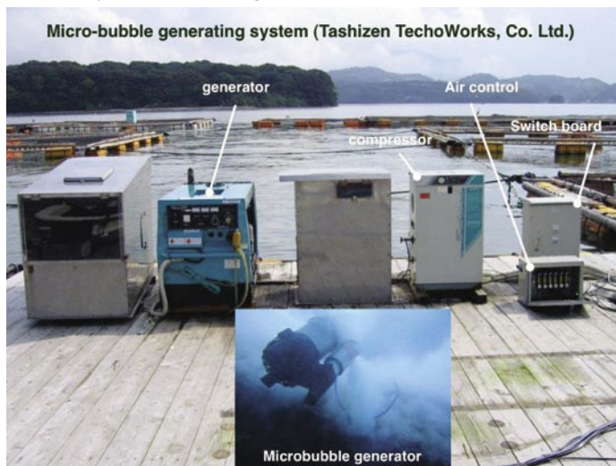
Figure 1. Micro-bubble generating system developed by Tashizen TechnoWorks Co., Ltd.
