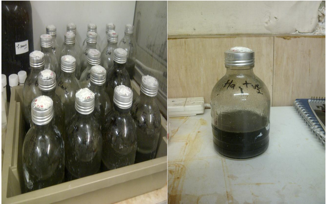
Fig. 2.3. Examples of reactor bottles (575ml) used for the batch assay, 300ml working volume was used leaving a 275ml headspace for gas analysis. Samples for analyses are taken from the top using syringes after gas measurement and then sealed with silicon material. Sampling was carried out every day for the first 10 days to monitor pH levels closely and was corrected when necessary. Gas volume measurements took into account changes in headspace volume over time.
