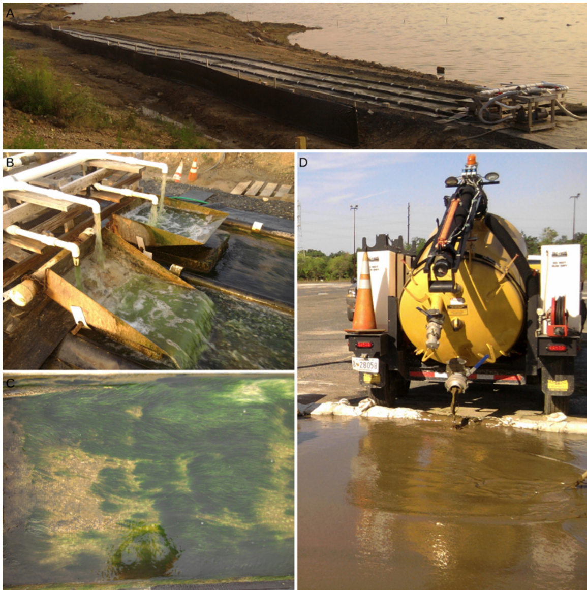
Fig. 1. Small-scale ATS. (A) A dual-flowway system, with each flowway 1 m × 100 m. Headworks are visible on the right. (B) Close-up of headworks, pulsing water into the system via tipping buckets. (C) Close-up of green filamentous algae ( Ulva ) growing in the flowway. (D) Harvested biomass vacuumed from the flowway being spread for solar drying.
