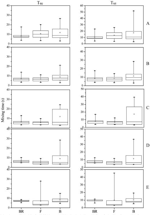
**Fig. 6** Mixing times at  $T_{90}$  and  $T_{95}$  for airlift bioreactor (BR), Fernbach (F) and balloon flasks (B) at five working flow rates: (A) 200; (B) 400; (C) 600; (D) 800 and (E) 1000 mL min<sup>-1</sup> ( $\pm$  S.D.)
