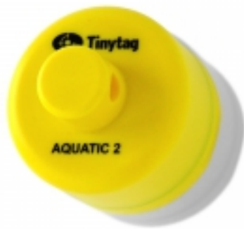
Figure 3.9. Tinytag® Aquatic 2 (TG-4100) temperature logger used to collect seawater temperature data at Ventry Harbour.
