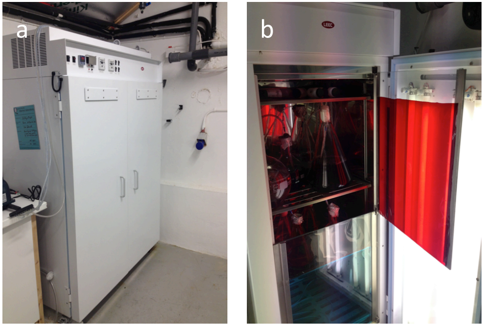
Figure 2.5 a) LEEC incubation cabinet external view and (b) Internal view with gametophyte cultures on shelves behind red light at QUB hatchery.
