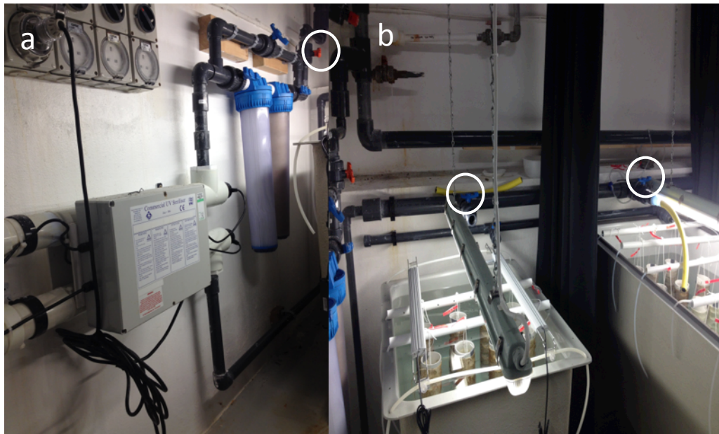
Figure 2.1. (a) UV sterilisation unit and double filters in housing. Inflow comes via the orange taps (circled) (b) First two tanks in a series of 5 supplied with water by blue taps behind (circled). The tubing below the water line is a fixed air-line.
