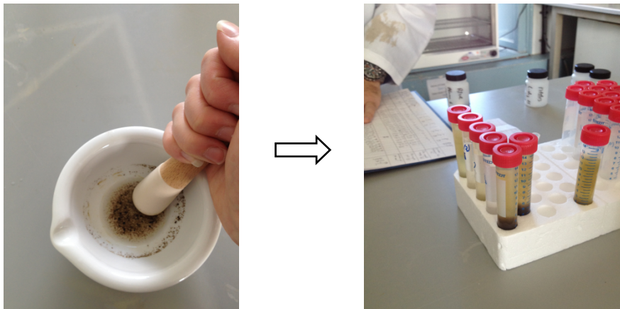
Figure 2.13. (a) Grinding the gametophyte clumps, and (b) transfer to Wintrobe tubes.
