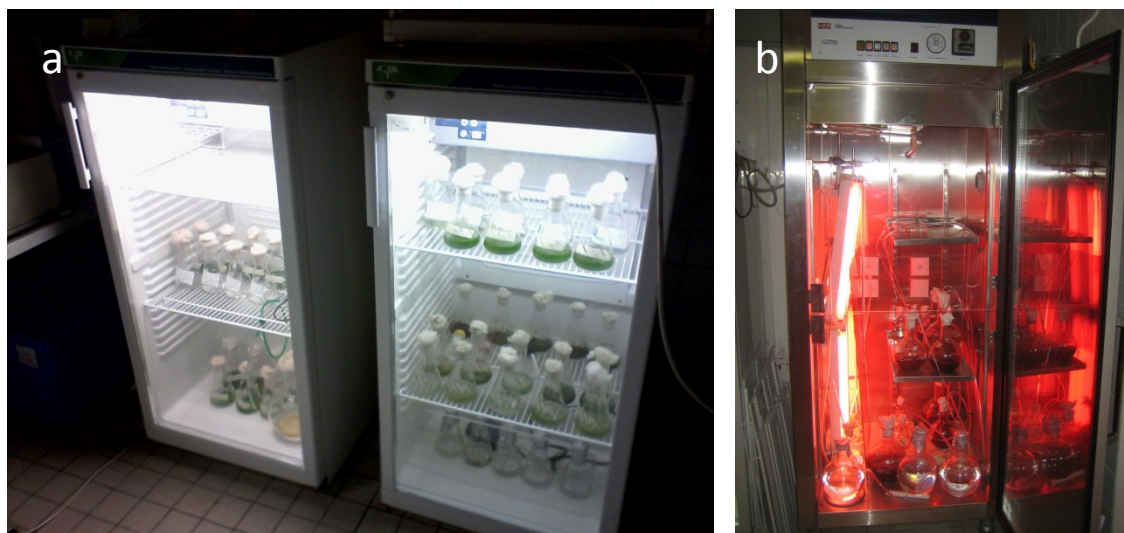
Figure 2.7 (a and b). Culture cabinets of 260L (a) and 500L (b), the latter being operated under red light for vegetative growth of Saccharina latissima gametophytes at the CEVA hatchery.
