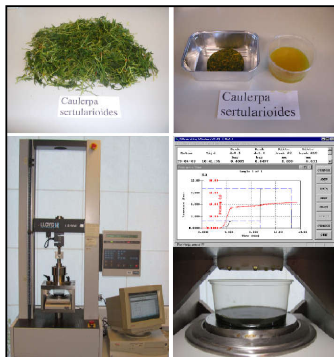
Fig.1. Pressure equipment to obtain press moisture from Caulerpa sertularioides
