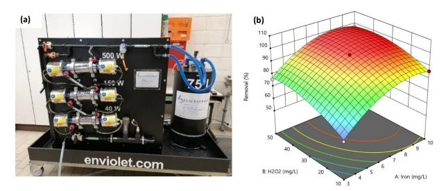
Fig. 10 (a) Photo-Fenton pilot system picture and (b) response surface of the system for indigo removal
