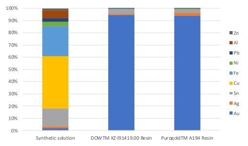
**Figure 18:** Metal composition (in %) of the initial multi-metal synthetic solution and the final Au solutions (eluates) after adsorption with DOW<sup>™</sup> XZ-I91419.00 and Purogold<sup>™</sup> A194 resins and elution with thiourea 0.1 mol/L and H<sub>2</sub>SO<sub>4</sub> 0.5 mol/L.
