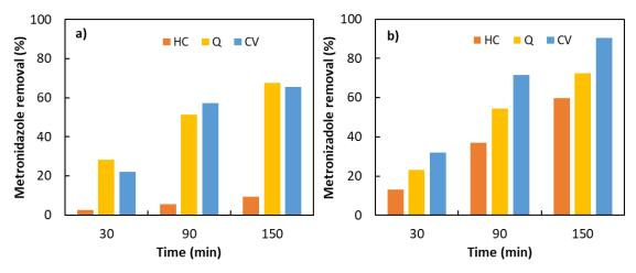
Figure 8: Metronidazole removal using different cathode materials by means of anodic oxidation (a) and homogeneous electro-Fenton (b)
