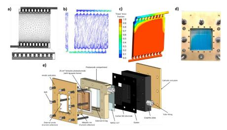
**Figure 15.** Details of the SolarFlow25 cell: a) mesh of the fluid body inside the cell, b) uniform upward electrolyte flow path lines generated at the central plane, c) and d) simulated vs experimental tracer test results (27 s after dye injection), e) exploded view of all cell components.
