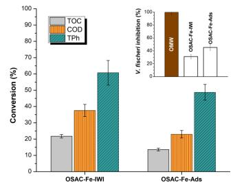
**Figure 19:** TOC, COD, TPh removal efficiencies for OSAC-Fe-IWI and OSAC-Fe-Ads catalysts (t = 240 min) and *V. fischeri* bioluminescence inhibition after 30 min of contact time with untreated and treated OMW samples (inset).
