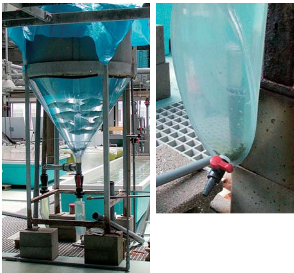
Fig. 2. The conical tank used to collect feces of fish fed the experimental diets to analyze nutritional absorption.
