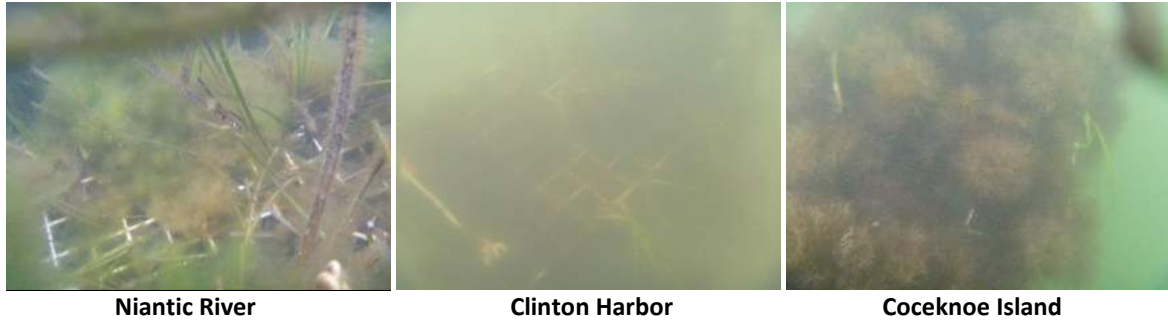
Figure 160: Images of NPI deployment rack on the retrieval day. Note that Niantic River eelgrass exhibits some filamentous green epiphytes, but eelgrass leaves are still visible. The turbidity at the Clinton Harbor site was high, leaves exhibited an epiphyte load similar to Niantic Bay, but the epiphytes were dominated by filamentous red algae. Cockenoe Island eelgrass leaves were almost completely hidden by the fine branching red algae (all algae present in the Cockenoe Island photo are attached to the eelgrass leaves or the deployment rack).
