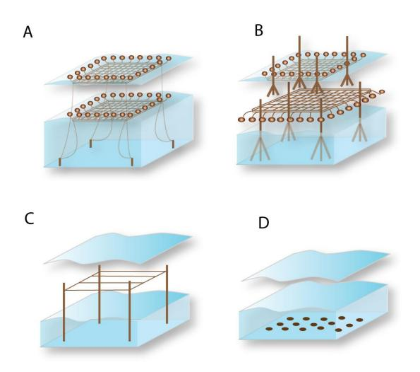
**Fig. 2.** Four basic types of seaplant agronomic methods. A. Floating raft in deep sea with deadweight mooring. Raft is floated all the time. B. Semi-floating raft in shallow water. Raft is floated at high tides but gets exposed during low tides. C. Off bottom in shallow water. Nets get immersed in high tide and exposed in low tide. D. Bottom planting in shallow water. Immersed at all the times. Water levels at high-tide are shown above low tide in all illustrations.
