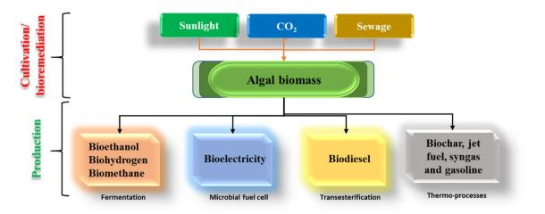
Fig. 5. Adapted: Production of various biofuels from algae biomass. Reproduced and modified from Saad et al. (2019) with permission.
