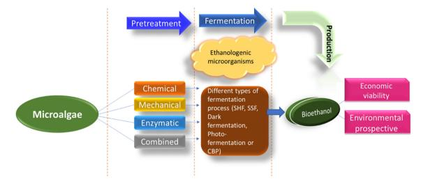
Fig. 7. Adapted: A general overview of bioethanol synthesis from microalgae using various pretreatments and fermentation methods. Reproduced and modified from Phwan et al. (2018) with permission.
