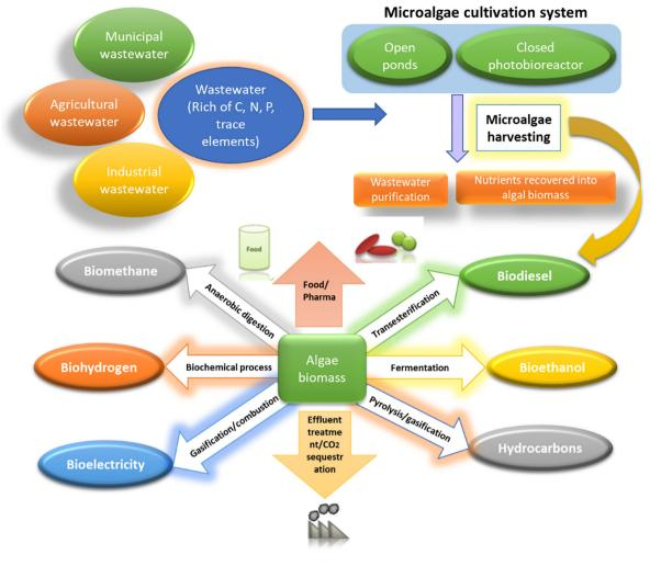
**Fig. 1.** Adapted: Wastewater remediation using microalgae and its application in various fields. Reproduced and modified from Aishvarya et al. (2015) and Liu and Hong (2021a) with permission.
