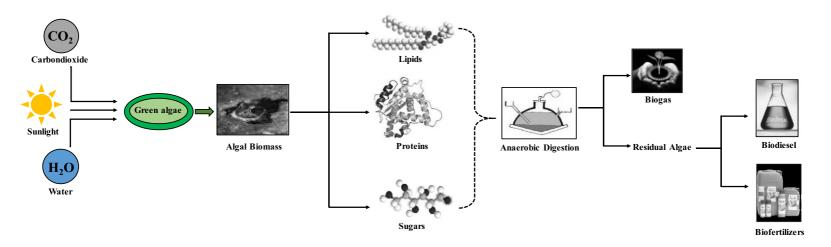
Fig. 3. Schematic representation of anaerobic digestion process for bio-valorization of algal biomass.
