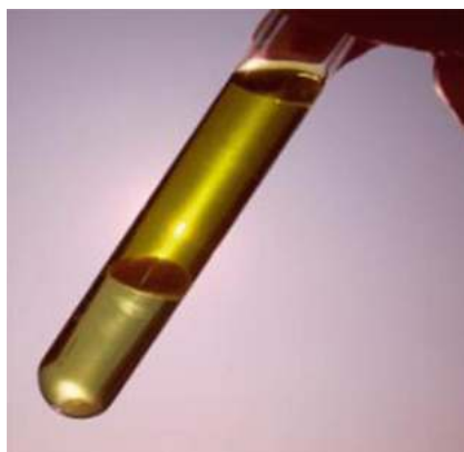
Fig. 8 Strategy for the extraction of hydrocarbons from B. braunii cultures by means of the switchable polarity solvent DBU/octanol
