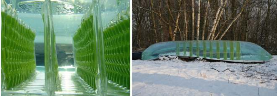
Fig. 8 Submerged flat panels in a Proviron photobioreactor [31]. Left : Floating reaction compartments in the inside of the reactor contain the algae suspension while the surrounding water serves mainly as temperature buffer and is equally important for the structure. Right : Exterior view at the reactor designed for outdoor applications
