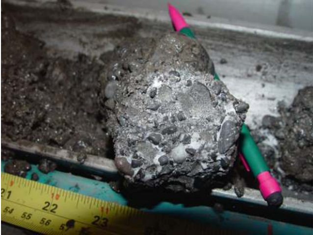
Fig. 5 Photograph of a gas-hydrate-bearing rock core from the Mallik 5L-38 gas hydrate research well. Note that the gas hydrate is the white material filling the void spaces in this conglomerate (photo courtesy of the Mallik 2002 Gas Hydrate Production Research Well Program [35])
