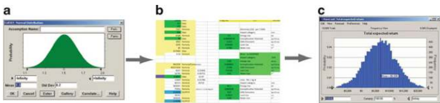
Fig. 4 Stochastic tools, such as Monte Carlo analysis, are receiving increasing attention from LC practitioners as means to systematically incorporate uncertainty into their analysis. Here, the process by which uncertainty in inputs is propagated through a spreadsheet model into empirical estimates of probabilistic output is demonstrated using screen shots from the CrystalBall Monte Carlo tool. (a) input distributions, (b) model, (c) stochastic outputs
